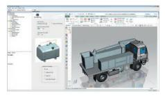
Using Rulestream facilitates the automatic generation of engineering work products, such as BOMs, CAD models, etc., according to design and manufacturing rules.
